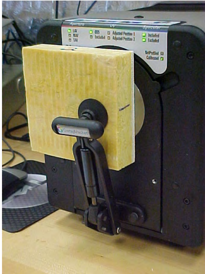
Photo No. 3 Light Reflectance Evaluation Showing Reading 1 in Process
